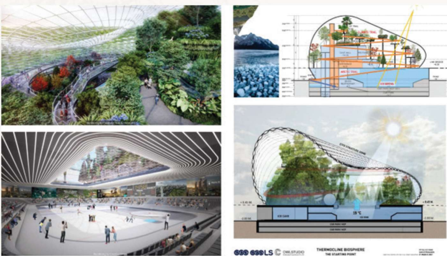
"Climaxias" Thermo-Active Dome with thermal air stratification design
