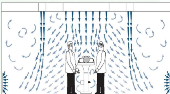
FIGURE 5: Laminar Flow System with Perimeter Air Curtain. Good protection of the patient from all sources of contaminants. Requires low to moderate air volumes.
